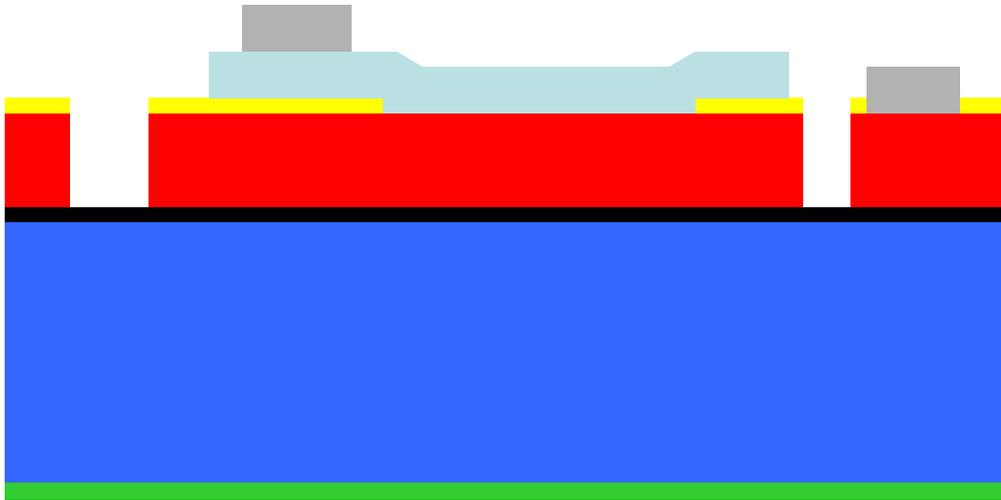
FIGURE 1.6. The wafers are coated with UV-sensitive photoresist and lithographically patterned by exposing the photoresist to UV light through the fourth level mask (SOI), and then developing it. The photoresist in exposed areas is removed, leaving behind a patterned photoresist mask for etching. The oxide layer is RIE etched. Deep reactive ion etching (DRIE) is used to etch the Silicon down to the Oxide layer. After etching, the photoresist is chemically stripped.
