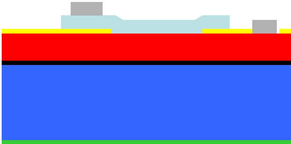
FIGURE 1.5. The wafers are coated with negative photoresist and lithographically patterned by exposing the photoresist with light through the third level mask (PADMETAL), and then developing it. A metal stack consisting of 20 nm chrome and 1000 nm aluminum is deposited over the photoresist pattern by beam evaporation. The photoresist is then dissolved to leave behind metal in the opened areas.
