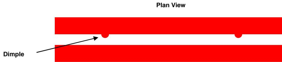
FIGURE 2.6.4. Example of dimple features in the SOI Mask level to reduce lateral stiction affects during release.
