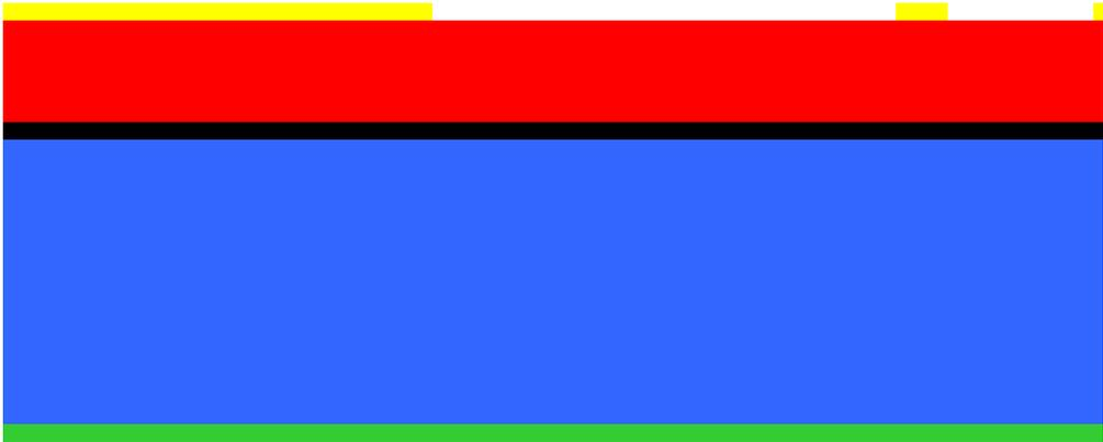
FIGURE 1.3. A 2000 Angstrom thermal oxide is grown. The wafers are then coated with positive photoresist and lithographically patterned by exposing the photoresist with light through the first level mask (PADOXIDE), and then developing it. The oxide is wet-etched. That is followed by an acid resist strip.
