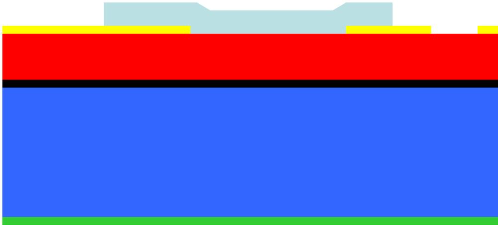
FIGURE 1.4. The film consisting of piezoelectric aluminum nitride is deposited over the wafers by reactive sputtering. The wafers are then coated with positive photoresist and lithographically patterned by exposing the photoresist with light through the second level mask (PZFILM), and then developing it. The material is wet-etched. That is followed by a solvent resist strip.
