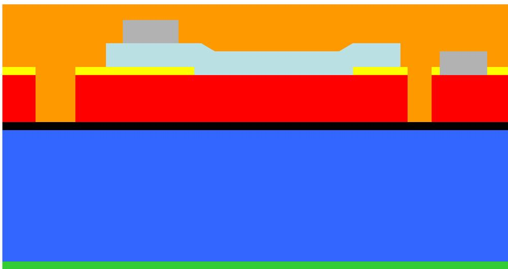
FIGURE 1.7. A front side protection material is applied to the top surface of the patterned Silicon layer. This is a polyimide coat that will hold the wafer together through subsequent trench etching.
